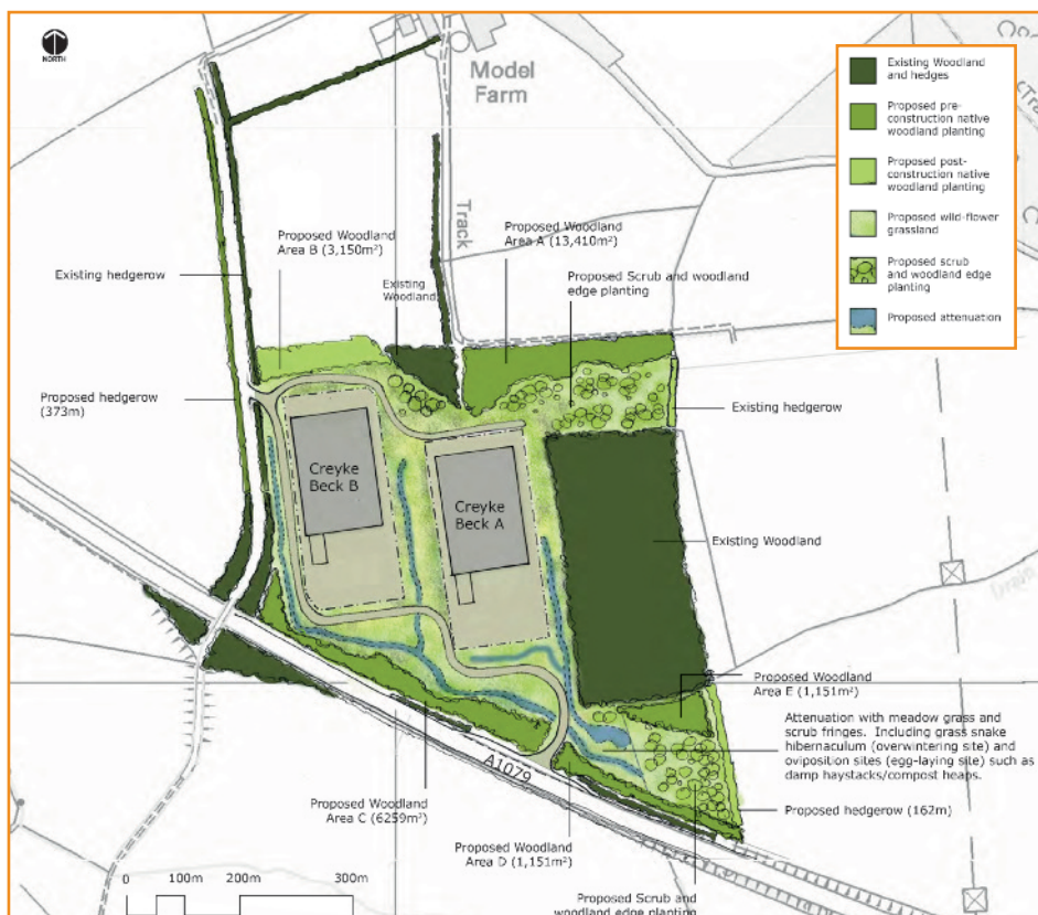
The proposed landscaping scheme for the Dogger Bank Creyke Beck converter station site
